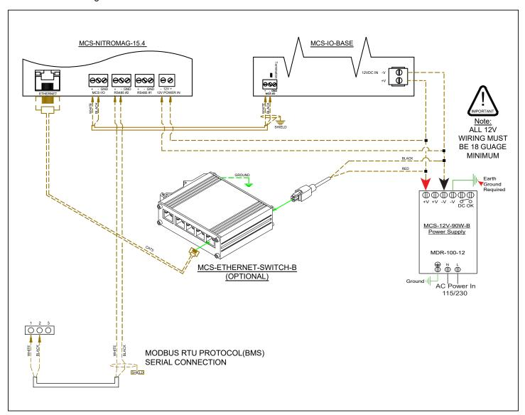
The MCS-NitroMag-N is configured through the MCS-CONFIG firmware. The MODBUS RTU MASTER supports up to 20 MODBUS devices e.g., VFD's, KW Meter, Compressors.
